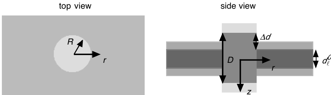
Figure 3.9: Schematic representation of the insertion of a hydrophobic rod with hydrophilic end caps in a bilayer.
