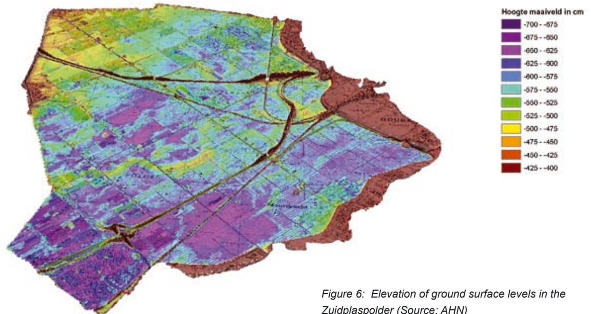
Figure 6: Elevation of ground surface levels in the Zuidplaspolder (Source: AHN)
