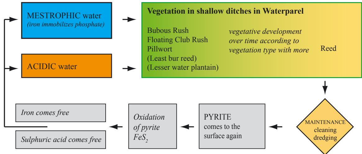
Figure 25: The 'pyrite-engine' in acid sulphate clay soil. With below right the 'ignition key' of the motor: maintenance.
