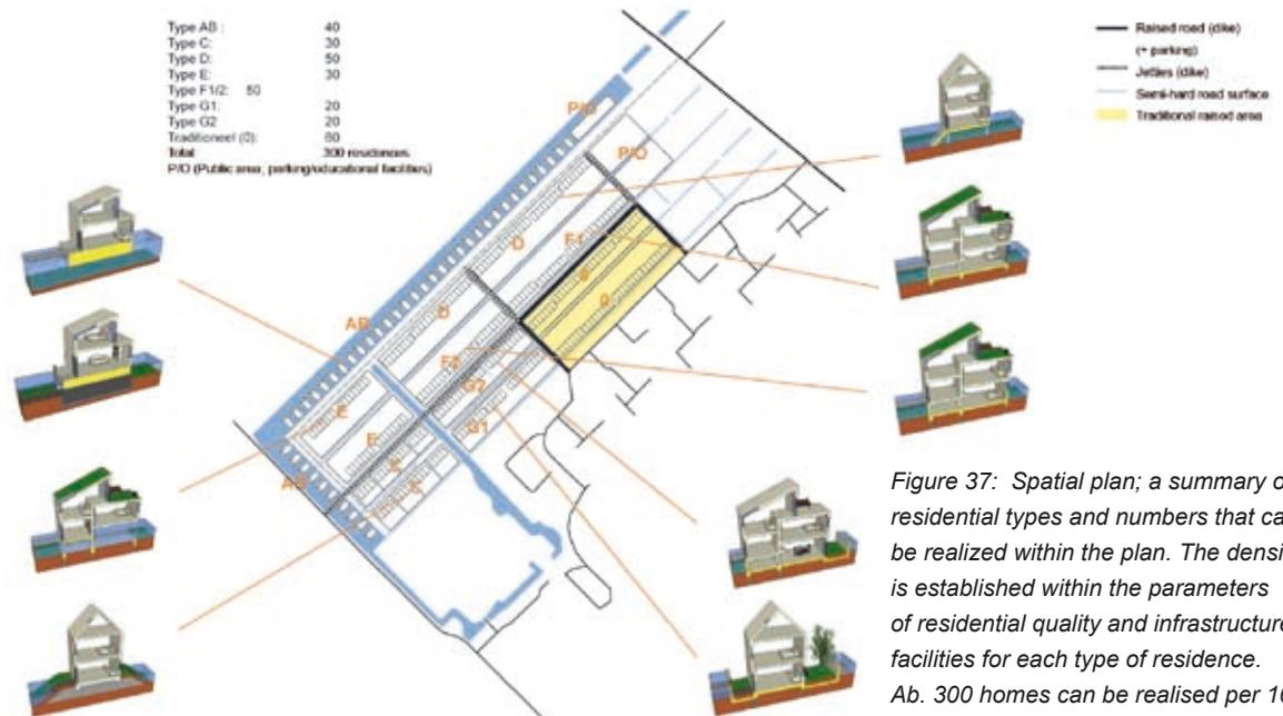
Figure 37: Spatial plan; a summary of residential types and numbers that can be realized within the plan. The density is established within the parameters of residential quality and infrastructure facilities for each type of residence. Ab. 300 homes can be realised per 10 hectares.
