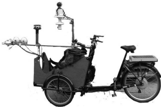
Figure 3: Cargo-bicycle equipped with micrometeorological measurement sensors
