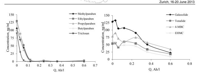
Figure 1. Electrochemical degradation of the personal care and household products which contain (left) and do not contain (right) phenolic ring.
