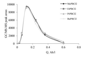
Figure 2. Formation of chlorinated parabens with increased specific electrical charge.
