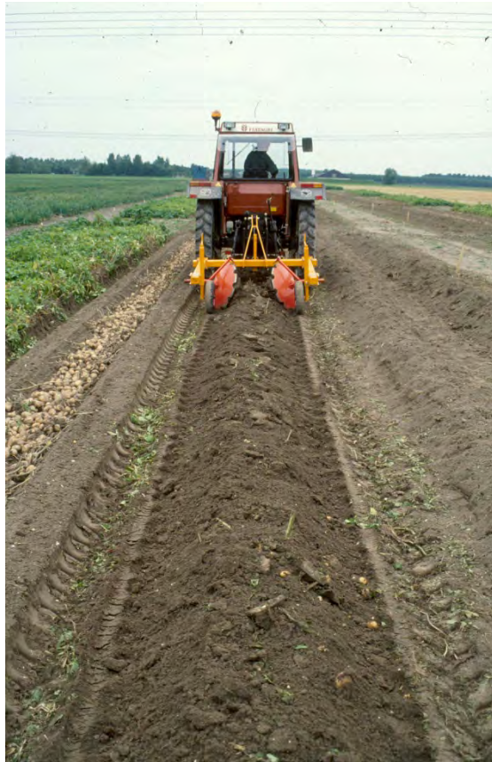
Picture 19. Lifter which is lifting two ridges and wich is putting the tubers in one row. Picture 20. Machine which is covering the lifted tubers with soil.
