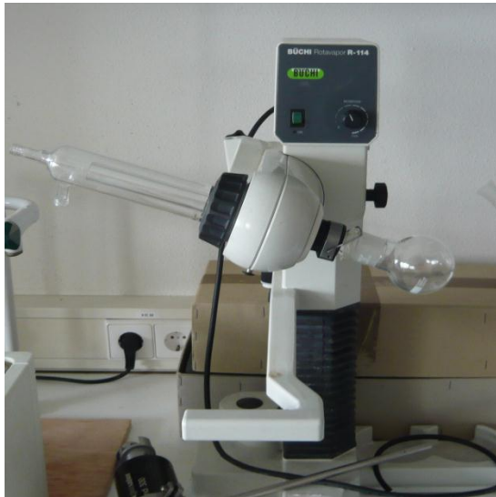
Rotary evaporator adapted for solid state polymerization
