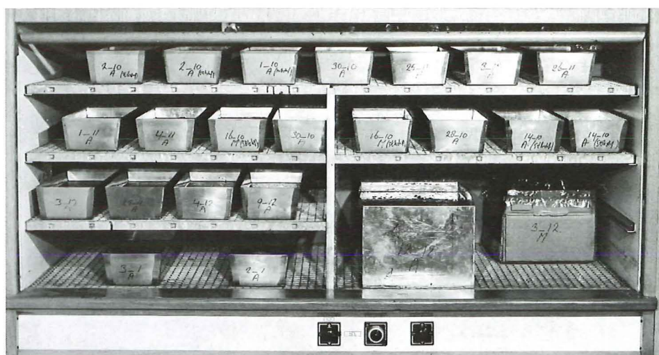
Fig. 9. Fume cupboard in which the temperature is kept constant at 20^{\circ}\text{C} \pm 0.5^{\circ}\text{C} . The boxes with impregnated samples are placed on grates in a continuous air stream. The two large boxes contain large impregnated samples which will be processed to mastodont-sized sections. The diluting agent in the left-hand box (steel!) is acetone, that in the right-hand one is monostyrene (a cardboard box lined with plastic foil).
