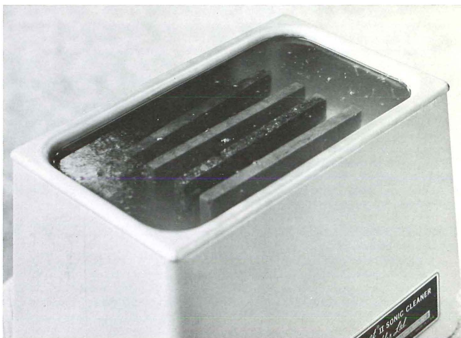
Fig. 16. Ultramet II Sonic Cleaner. The cleaning liquid is petrol.
