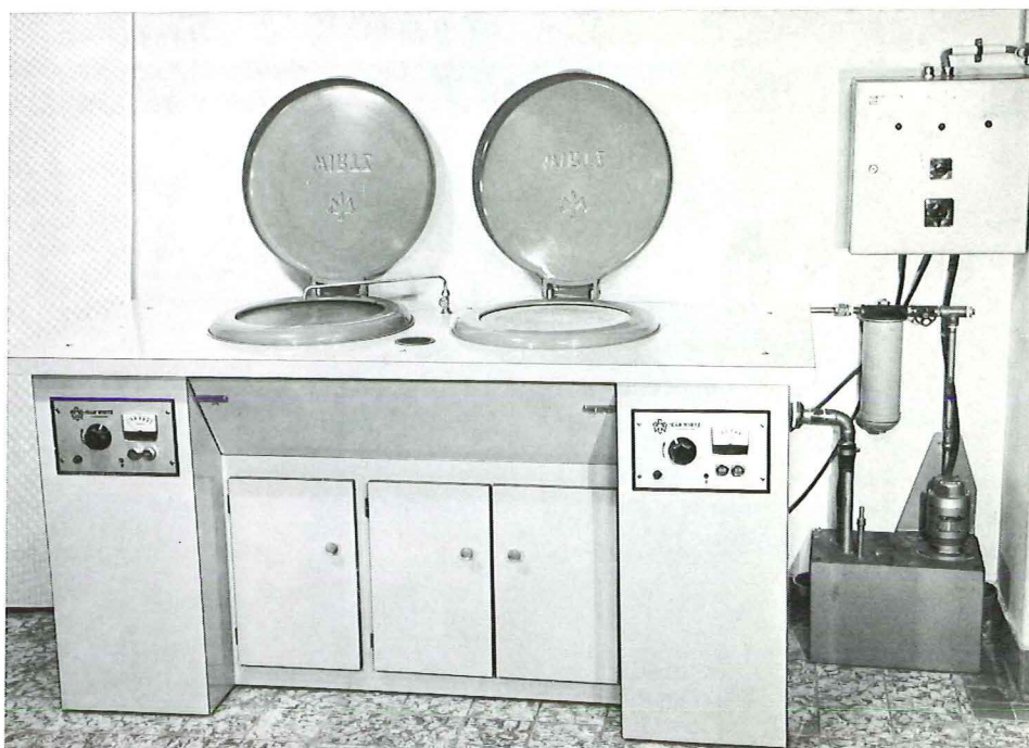
Fig. 19. A Wirtz machine for fine grinding and polishing. The machine is equipped with rotating Triefus discs of 350 mm diameter. The speed of the left-hand disc can be varied from 0 – 250 r.p.m., that of the right-hand one from 0 – 500 r.p.m. Discs for fine grinding consist of diamond impregnated synthetic material, and a copper disc is used for polishing.
