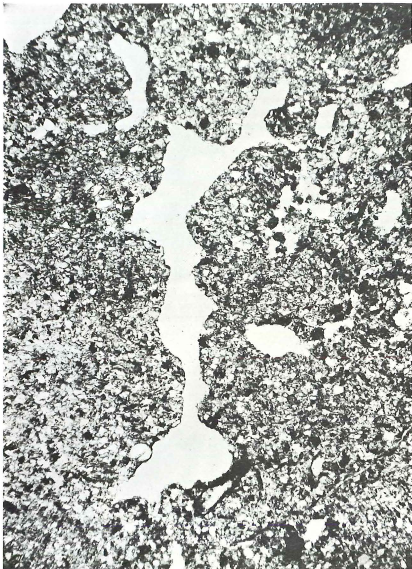
Fig. 69 Organo-mineral excrements (bacillocylinders) of earthworms. By "ageing" the excrements will amalgamate together. After a certain period only the uneven wall of the void will betray their earlier presence. Thin section in plain light, 40 x.
