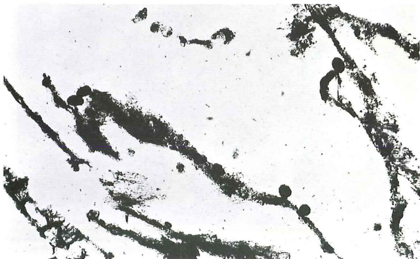
Fig. 43 Sporadic basic distribution pattern of fine, organic ellipsoids. Thin section in plain light. 37 x.
