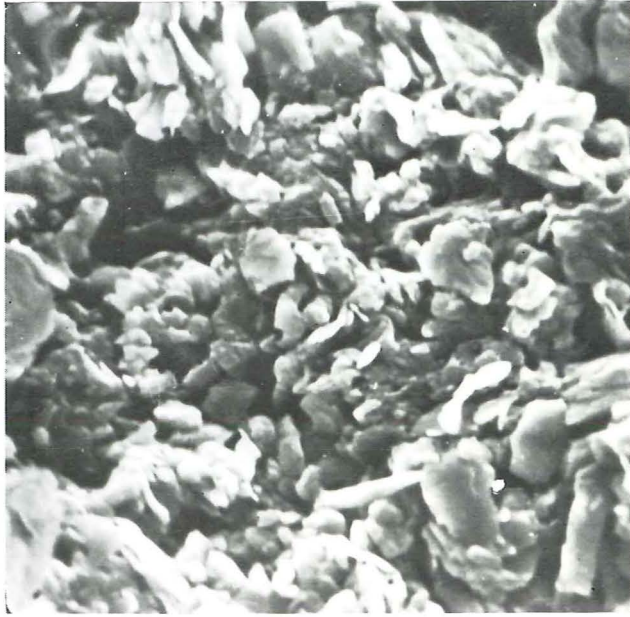
Fig. 13 Detail of Fig. 12. The extremely small particles of approximately 2\mu\text{m} are remnants of cellwalls. They represent a particular group of organic plasma. 5154 x.
