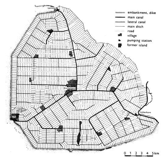
Fig. 8. General lay out of the Northeast-polder.
