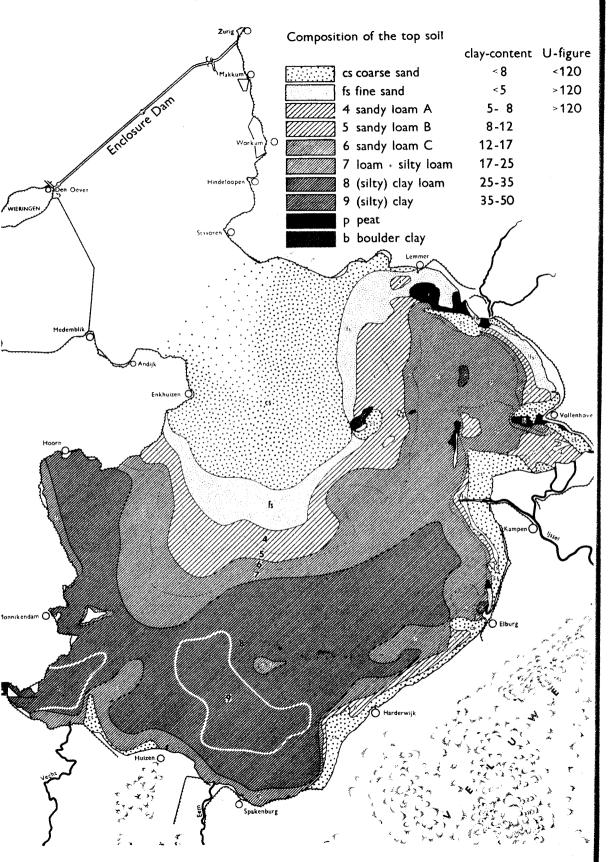
Fig. 6. Soil map of the Yssel-Lake as a result of the under-water survey.
