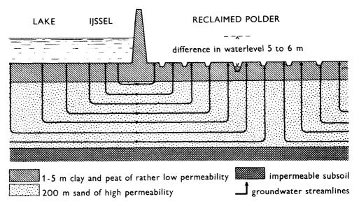
Fig. 7. Seepage into the Yssel-Lake polders (schematically).
