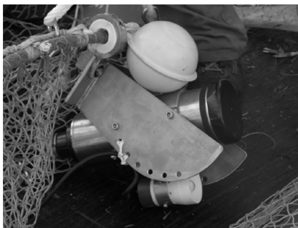
Figure 12. Headline camera used by IPIMAR; from: (ICES, 2007).
