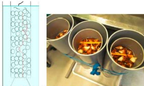
Figure 1. Experimental setup to assess suspected bulb lots for the presence of Ditylenchus dipsaci . To trace the nematode specific conditions are required to reduce the influence of rest material in the samples to be tested.
