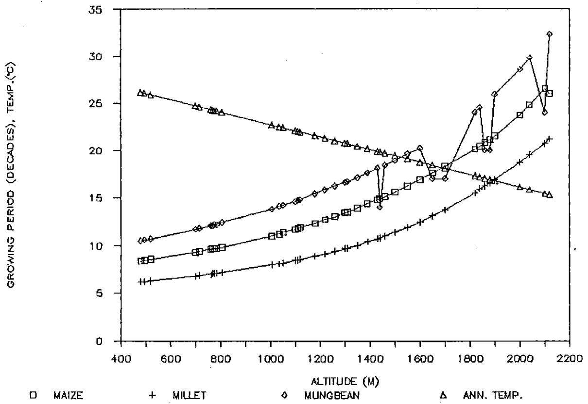
Figure 14. Relation between altitude and the length of the growing period for maize, millet and mungbean when emerged at the 10th decade.
