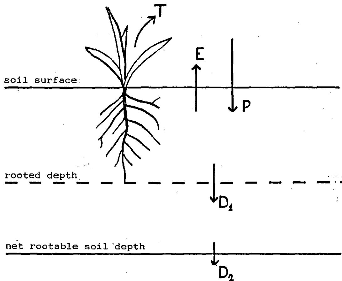
Figure 5. Soil layers and moisture flows in the model. E = evaporation from the upper soil, P = precipitation, D1 = drainage of rooted layer to subsoil, D2 = drainage out of the subsoil.
