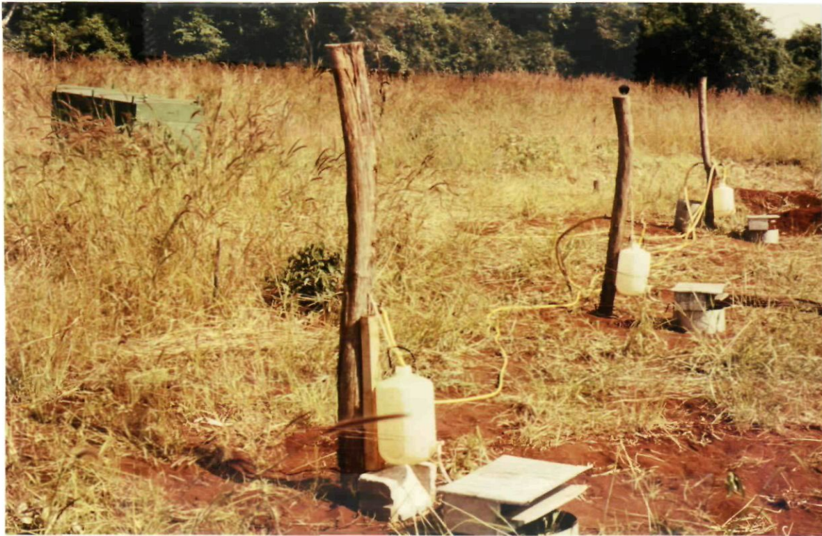
Photo 5.5. Lay-out of the leaching trial. The water-tank was placed upslope to create water pressure. For further explanation is referred to Figure 5.2 (WL81).
