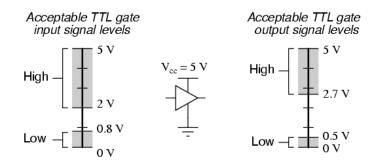
Figure 2. Transistor-Transistor Logic signal levels for input and output signals.
