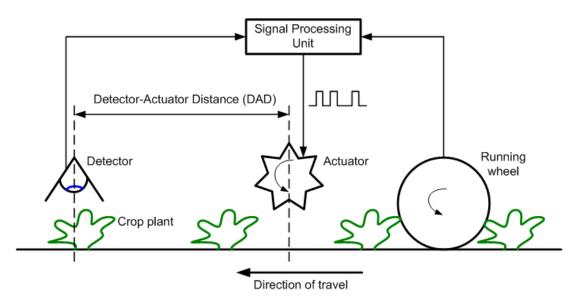
*Figure 1. Schematic lay-out of a machine for intra-row weed control defining the Detector-Actuator Distance* (DAD).
