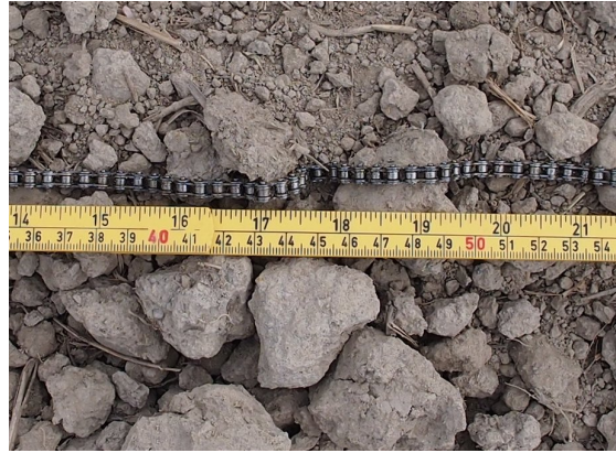
Figure 6.4: Picture from measuring soil roughness with a chain. From the fieldwork. Photo by: L. Thomsen
