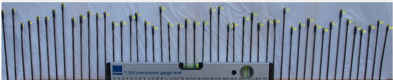
Figure 6.3: Screen-dump from the image processing program. Using the ruler in the image a Cartesian coordinate system covering the picture was created with origin in the upper left corner. Then each tip of pin was digitalized manually and a text file with the coordinates was exported to Excel for further processing.
