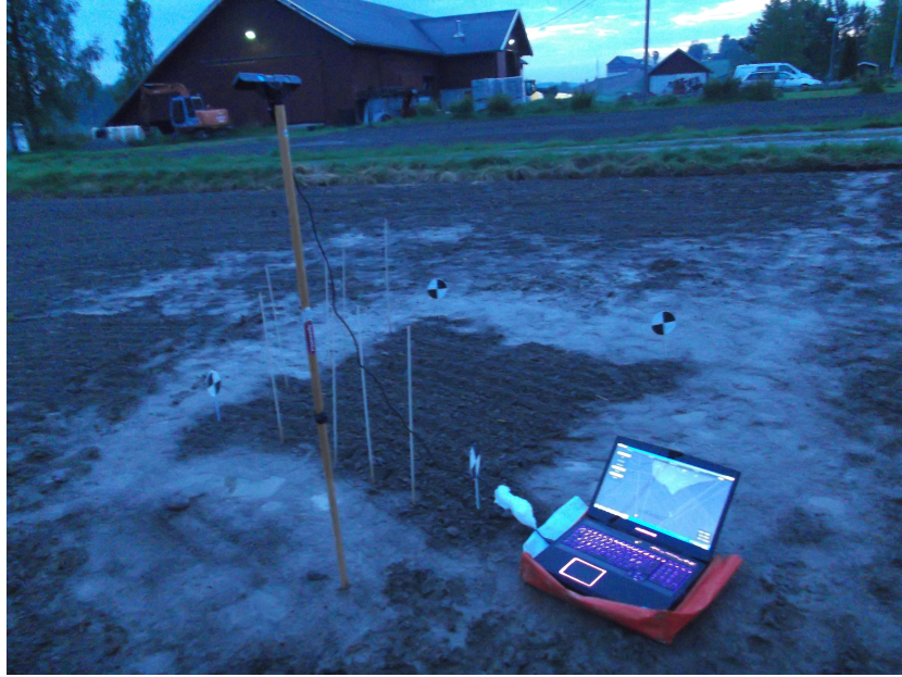
Figure 6.10: Data acquisition with the Xtion during late in the evening. The Xtion is mounted on a wooden stick and is connected to a laptop. Photo by: L. Thomsen
