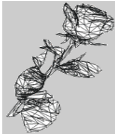
Figure 6. A wireframe model of a rose, scanned with 3D scanning equipment.
