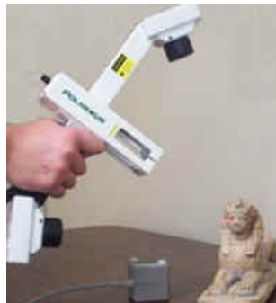
Hand-held laser scanner (left) and the produced image (right). Notice the different positions of the light source and the receptor, in order to detect laser shifts by the triangulation method.
