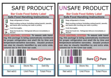
**Figure 1.4** Example of a biosensor from Food Sentinel System™ (SIRA Technologies, California, USA) that results in unreadable barcode in case of food safety risk.
