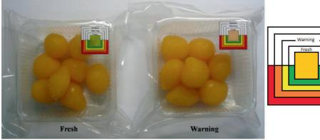
Figure 1.3 A sensor that monitors carbon dioxide as indication for the freshness of the dessert golden drop (Nopwinyuwong et al., 2010).
