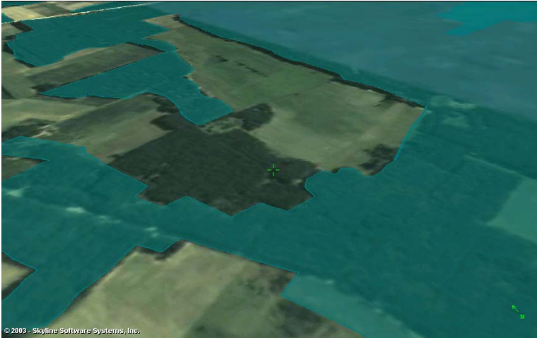
Fig.50 Comparison of boundaries of the forest: aerial photograph and vector layer made based on topographical map.
