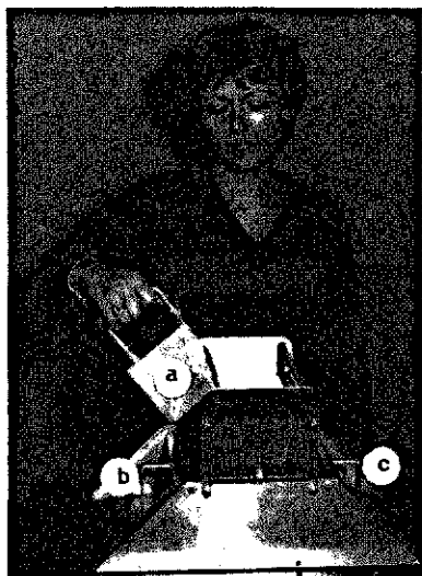
Figure 8. Soil divider. The first of a series of halvings is shown.
