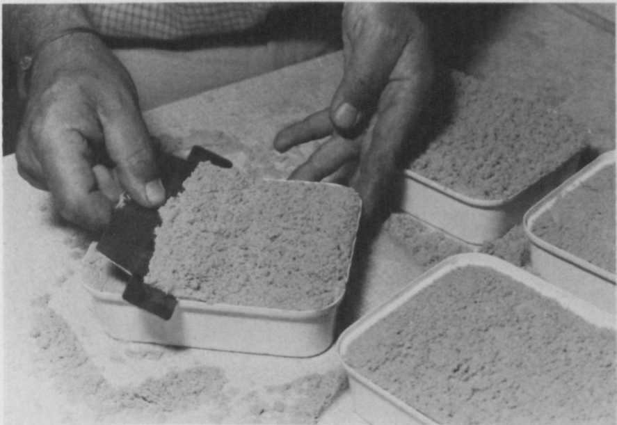
Figure 36. Excess of sand is removed with short side of the scraper.
