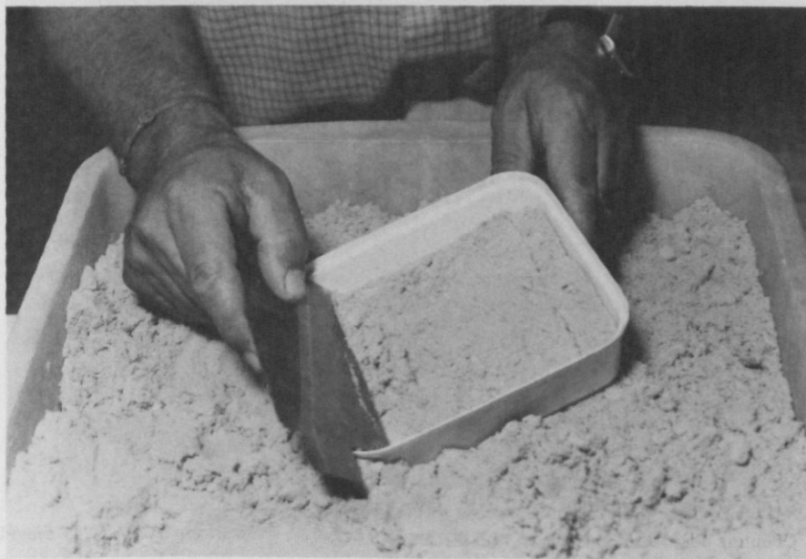
Figure 28. Container is filled with moist sand and levelled with the long side of the scraper.
