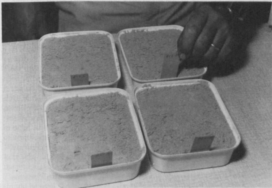
Figure 37. Slips with analysis number are inserted in beds.
