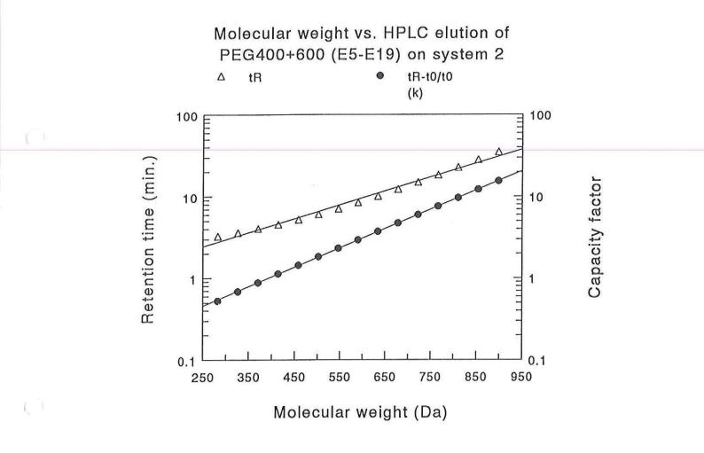
ANNEX 6. Calibration curves for oligomers E5-E9 of a mixture of PEG400 and PEG600 in the range of 0.1 - 3 mg PEG[400+600] mg/ml.
