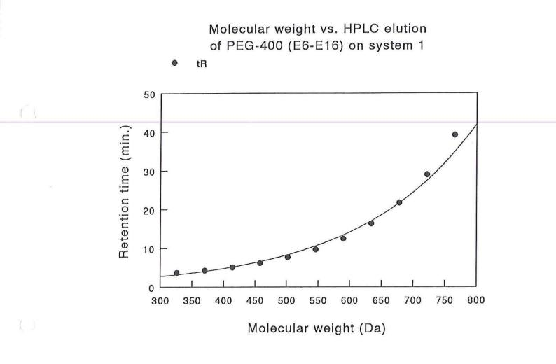
ANNEX 4. Log-linear relationship between molecular weight and capacity factors of oligomers of PEG400 (E6-E16) on HPLC system 1.
