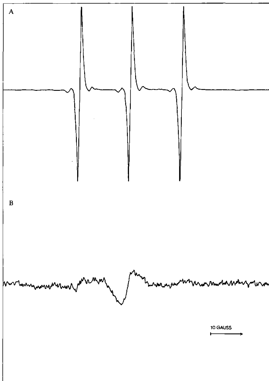
FIG. 5.7. EPR spectra of the maleimide spin label. (A) 27 \mu\text{M} label in 0.05 \text{ M} Tris-HCl (pH 7.1). (B) the label aspecifically bound to PDC (protein concentration 3 \text{ mg ml}^{-1} ). Binding is the result of incubating 9 \text{ mg} PDC with 90 \text{ nmoles} spin label in 0.05 \text{ M} Tris-HCl (pH 7.1) in a volume of 0.3 \text{ ml} during 3 \text{ min.} at 20^\circ . The reaction was stopped by eluting the mixture through a Sephadex G25 column with 0.05 \text{ M} Tris-HCl (pH 7.1). EPR conditions: temperature, 20^\circ ; scanning rate, 6 \text{ gauss min}^{-1} ; time constant, 3 \text{ sec.} ; frequency, 9458 \text{ GHz} ; modulation amplitude, 1 \text{ gauss} ; gain, (A) 10^5 (B) 10^6 .
