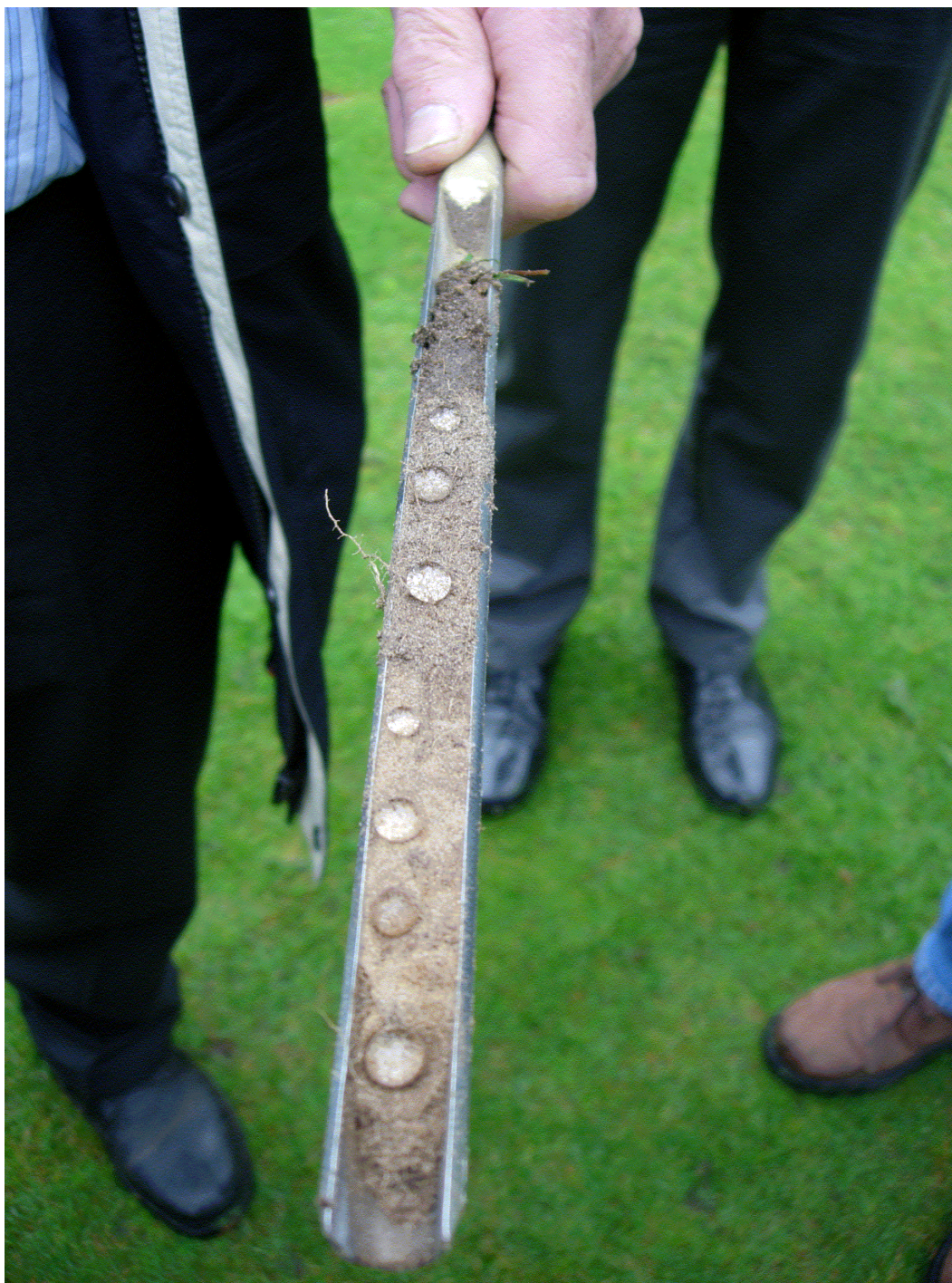
Figure 3.14 Determination of the occurrence, depth and thickness of a water repellent layer in the field, by using a small core sampler.
