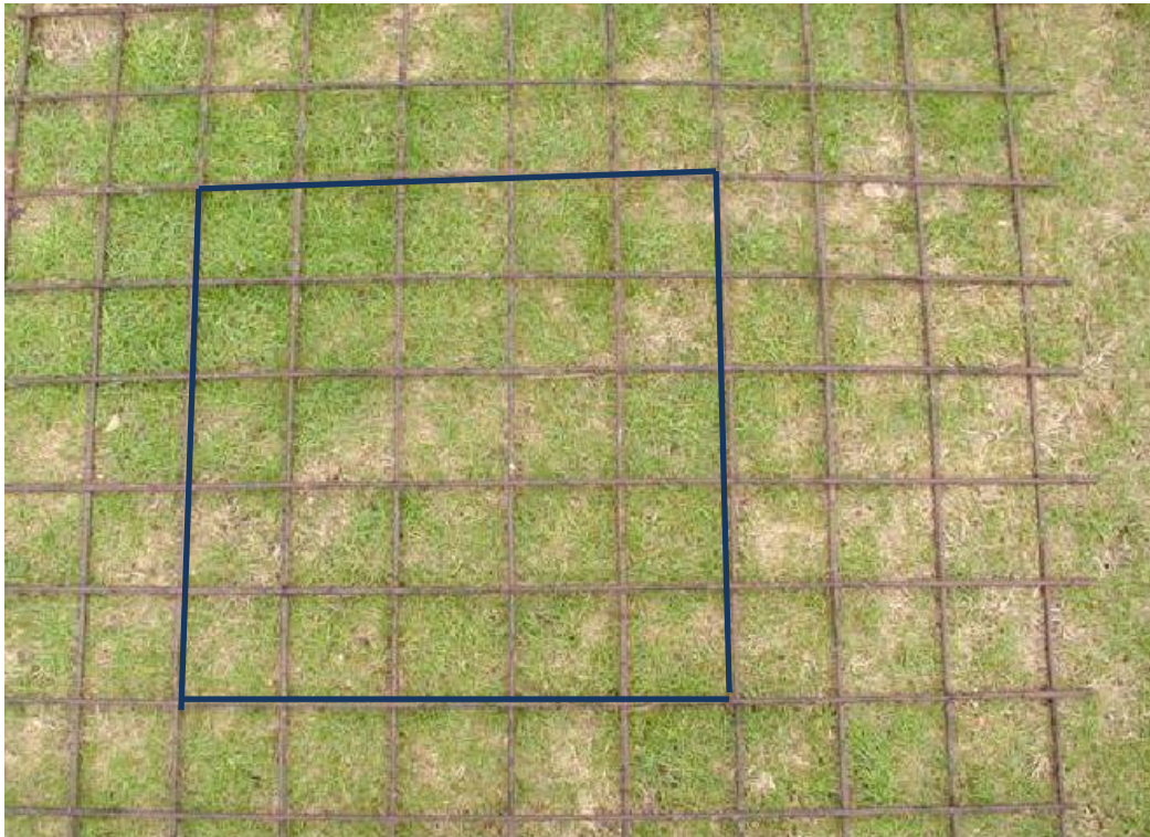
Figure 2.3 Estimation of the percentage green grass in adjacent compartments, squares of 10 cm by 10 cm, by using an iron grid of 1 m by 1 m.
