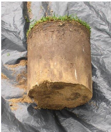
Figure 2.6 Taking the soil columns in the experimental plots with the cup-cutter to a depth of 18 cm, and refilling the holes with columns from a nursery.
