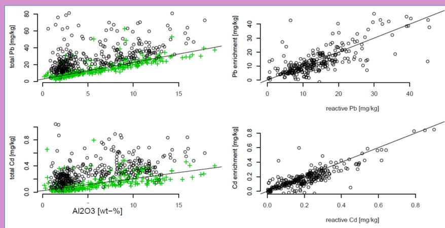
**Figure 1. (Left)** Geochemical baseline model of metal vs Al<sub>2</sub>O<sub>3</sub> in subsoil (green symbols and regression line) to estimate topsoil enrichments (black circles). **(Right)** Reactive metal concentrations (0.43 HNO<sub>3</sub>-extractable metal concentrations) vs estimated enrichments. The line depicts the 1:1 relation.
