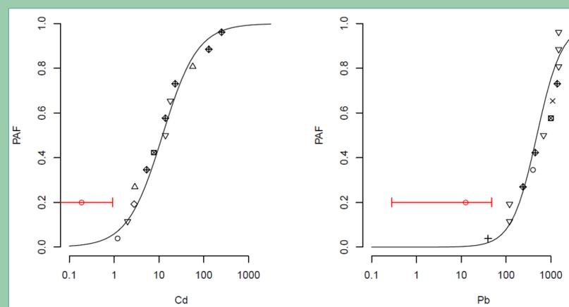
**Figure 3.** Species Sensitivity Distributions for Cd and Pb, based on chronic ecotoxicity data from Crommentuijn et al. (1997). The red horizontal lines refer to the X-axis only and indicate the ranges (minimum, maximum) of the measured reactive concentrations in Dutch topsoils (red circles are median values).
