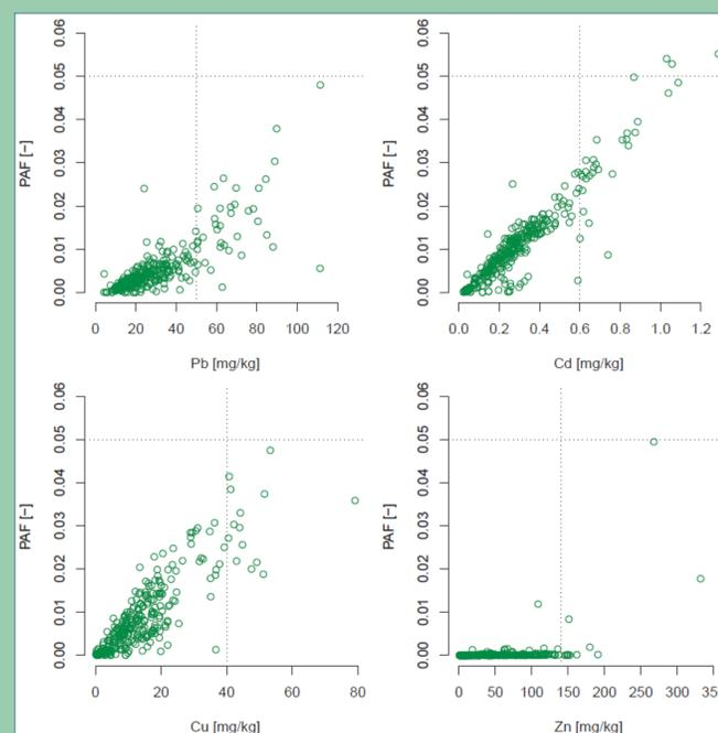
**Figure 4.** Total soil concentrations and toxic pressures (PAFs based on the reactive concentrations in the same samples). The horizontal lines depict the regulatory HC<sub>5</sub> value, as derived from ecotoxicity tests with species, the vertical line depicts the soil threshold value.
