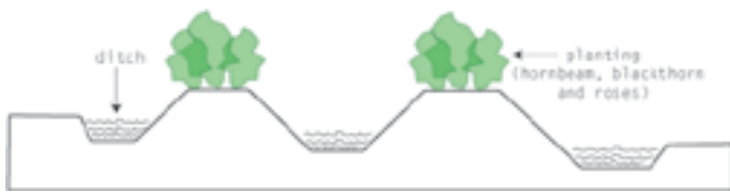
3.15 Section of planting on a 'landweer' (Adapted from Boosten et al. 2012)
