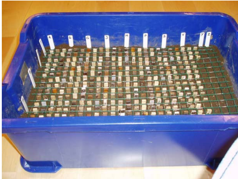
Figure 6: Test set-up for TMC test (ENV 807), illustrated by the soil box with soil from the old Simlångsdalen test field.
