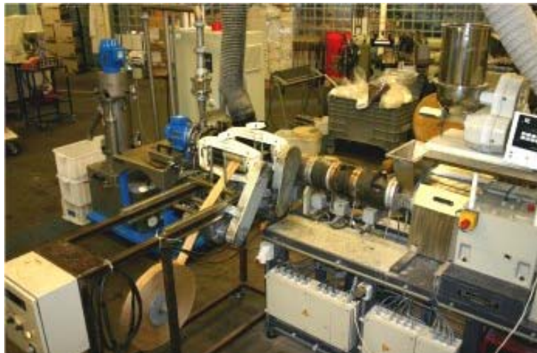
Figure 1: Extrusion compounding facility at A&F used for compounding of furfurylated wood particle-PLA WPC material.
