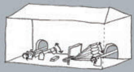
The driveshaft connected to the water wheel then powered the bellows and hammers used in the iron production.
