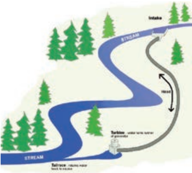
[11.14] Sketch of micro hydro power installation. It shows similarities to the classis Ferrerías.
