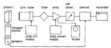
FIG. 5. Block diagram of amplifier-demodulator. Prism 1 is  $P_1$  of fig. 3.
