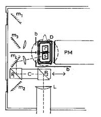
FIG. 11. Adaptation of the scattered transmission accessory of the Cary-14 spectrophotometer to irradiation of sample s inside a cryostat. D: cross section of dewar flask (see fig. 12). The 90° prisms P<sub>1</sub> and P<sub>2</sub> are mounted together on a carriage C. During spectrum recording, this carriage is slid out of the measuring beam. b: Baffles. r: reference sample, receiving no actinic irradiation.
