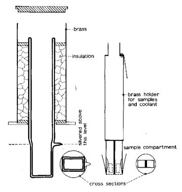
FIG. 12. Liquid nitrogen dewar for measurements at low temperature. In the lower part of the vacuum flask, of rectangular cross section, apertures are left unsilvered for admission of the beams. The coolant is introduced into the brass sample holder (right) and samples are cooled by conduction. There is no coolant in the light path. A thermocouple is soldered to the lower edge of the sample compartment in order to measure the temperature inside the cryostat (not shown).
