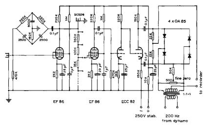
FIG. 6. Circuit diagram of the amplifier with 200 Hz filter section and ring demodulator. A symmetrical low pass filter is inserted between the amplifier output and the potentiometer to remove any 200 Hz that may appear at the output terminals.
