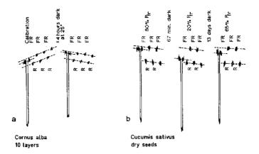
FtG. 14. Examples of phytochrome measurements, made with the dual purpose instrument, described under section 4. Two-wavelength mode, 730-806 nm. After writing a calibration mark, the traces were recorded during 30 sec each, with alternate exposures of the sample to actinic red (R) or far red (FR) light for 45 or 60 sec. Upward movement: increased absorption at 730 nm relative to 806 nm.
