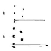
FIG. 15. Effect of beam intensity upon signal to noise ratio. Both recordings with same sample (white paper). In experiment b, the light intensity of the measuring and reference beams was about 10 times that in experiment a, the amplification having been adjusted to give roughly the same signal. This experiment shows that the noise is due to shot noise of the photomultiplier.
