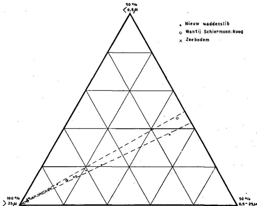
Fig. 7. New „Wadden” mud (•), wan-tide (o) and sea-bottom (x) samples
