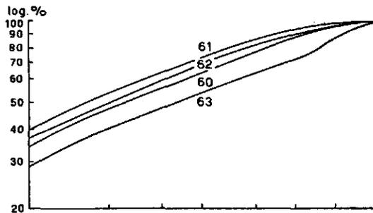
Fig. 5a. Mud from sea-water (logarithmic cumulative curves)
