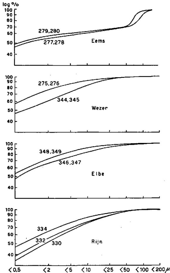
Fig. 6a. Mud from river-water (logarithmic cumulative curves)
