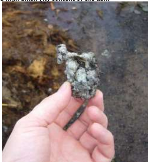
Figure 9. Example of ash agglomeration formed due to a low ash melting point in boilers due to a high alkali (K) content of the ash.
