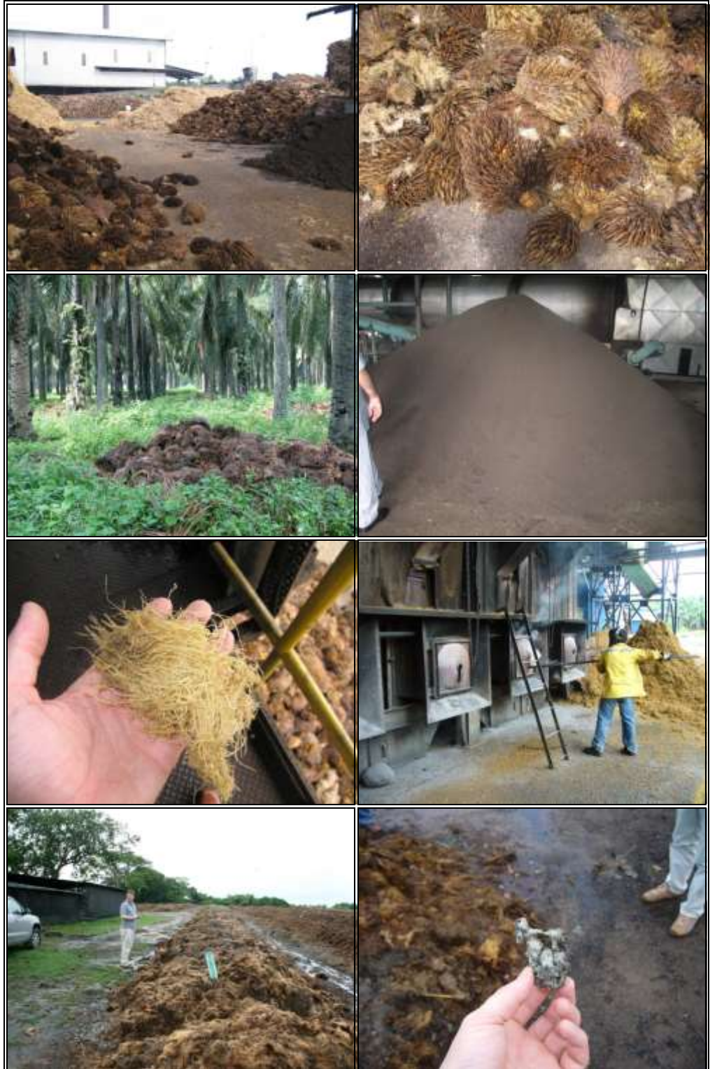
Figure 7. Mill byproducts are stored near the mill. EFB is mainly returned to the plantation and mulched or burned to produce bunch ash. Fibre is mainly used to provide energy for steam generation. In some cases compost is produced from EFB and fibre and ash. (Pictures taken at Agro Palma S.A. Brazil; Daabon, Colombia; and Malaysia).
