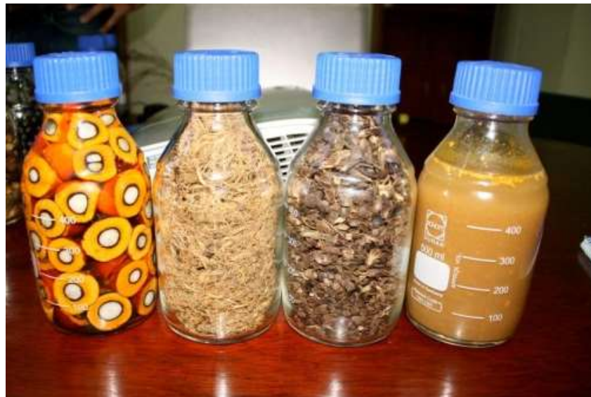
Figure A. Palm fruit is processed into oil and by-products (mesocarp) fibre, shell and POME (palm oil mill effluent).
