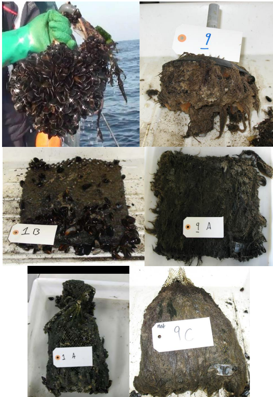
Figure 7. Examples of collectors after retrieval from the first week of deployment (left) and the ninth week of deployment (right). Top: Chinese hats, Middle: Vexar mesh, Bottom: Mussel stockings.
