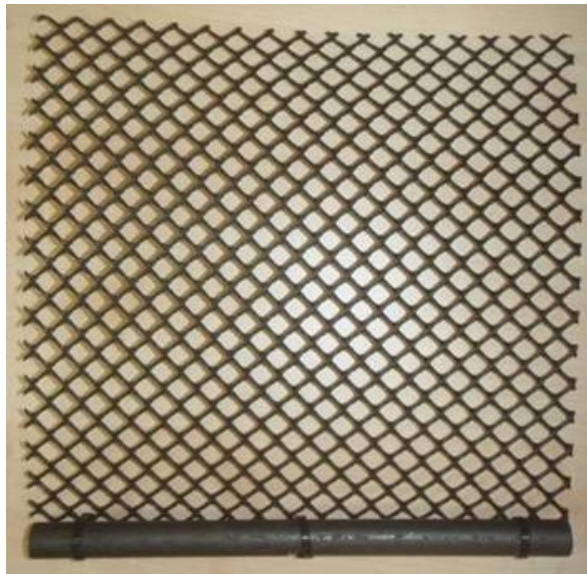
Figure 2. Prepared 30 x 30 cm square of Vexar mesh with attached steel rod used in the Netherlands. One square was one replicate in the experiment.
