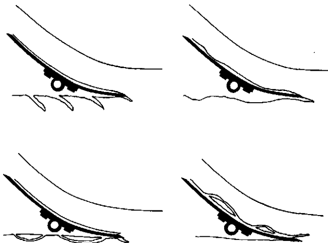
FIG. 11. Tongues, holes and slices in the case of intake with open crack formation.
