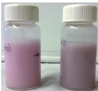
Figure 4.9 Alginate nanospheres containing 0.001% Congo red dispersed in MCT oil. Left sample is an emulsion of alginate solution in oil (no \text{CaCl}_2 added) and in the right sample \text{CaCl}_2 nanoparticles have been added.
