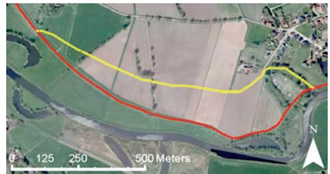
**Fig. 2. The draft design of the floodplain restoration measure involves dyke realignment, land use change (agriculture to nature) in the German part of the study area and increased meandering in the Dutch part of the study area. The indicated realignment – from red (current) to yellow (future situation) – is hypothetical.**
