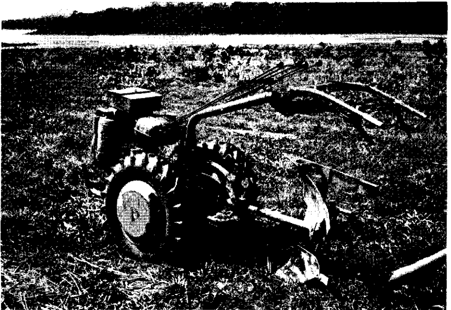
FIG. 7. Heavy two-wheel tractor (7.4 kW).
