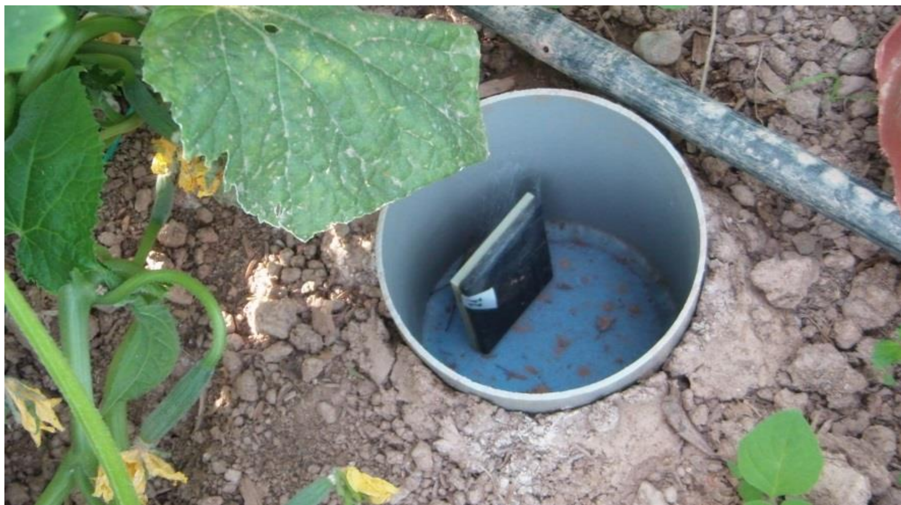
Figure 2. The AquaTag placed in a PVC jacket with a cucumber cultivation.
