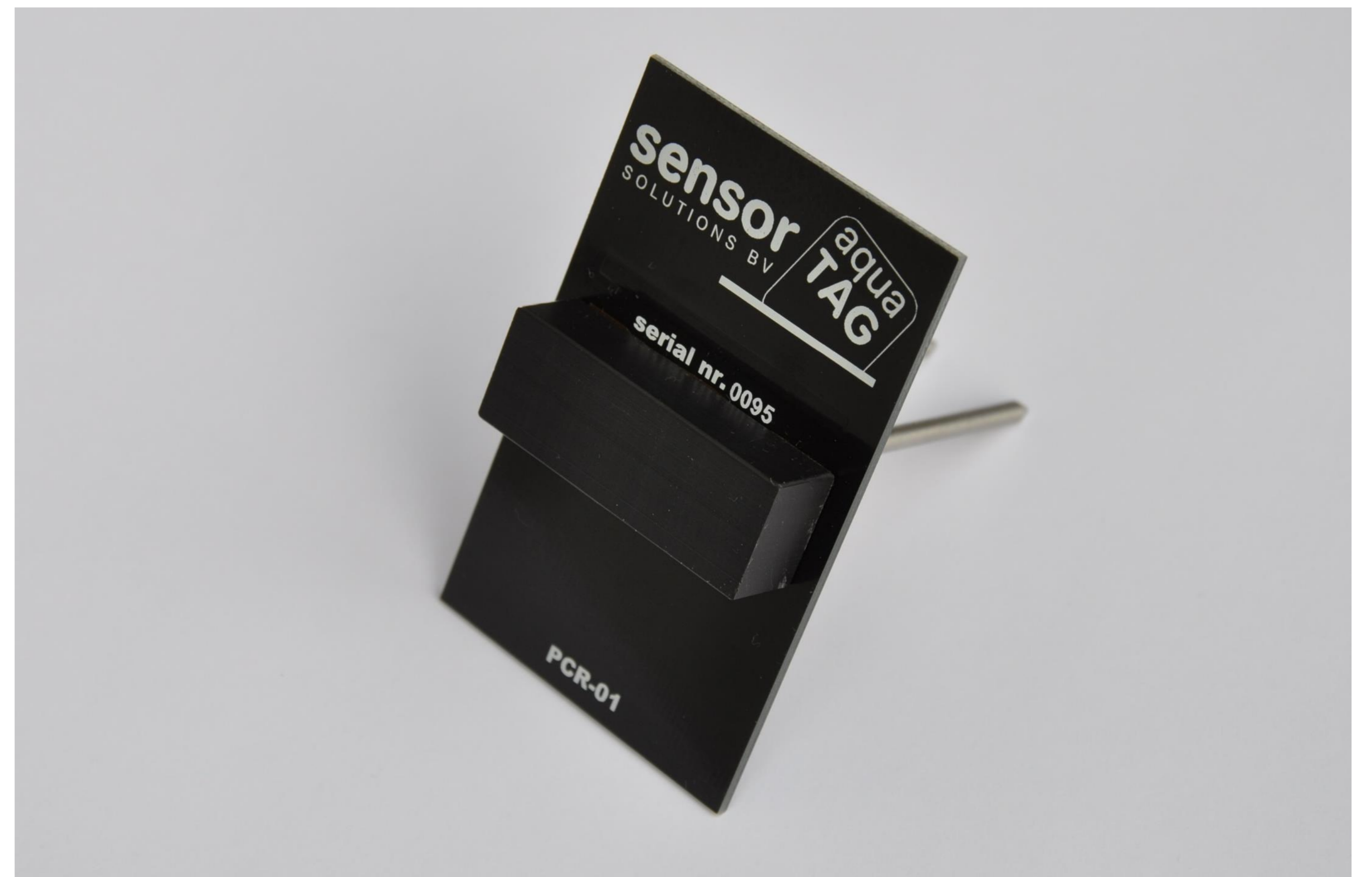
Figure 1. The AquaTag (version especially for container plants).
