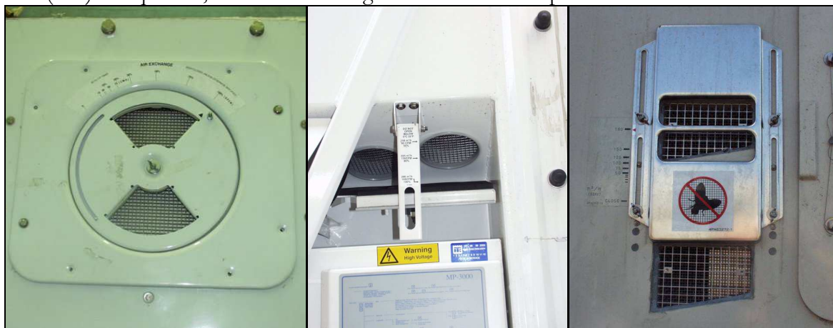
Fig. 15, some of the most common fresh air vents (from left to right Carrier, Thermo King and Daikin).
