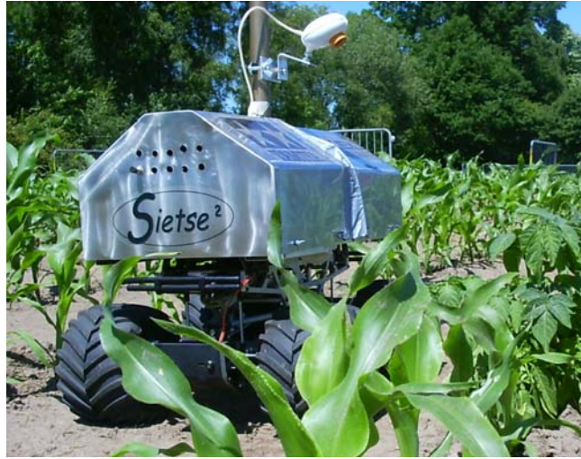
Fig. 1. This experimental robot was used in field tests of the detection method for broad-leaved dock.
