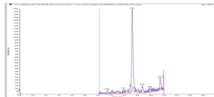
Combined chromatogram of blank (red) and spiked sample 5 µg PHA/kg (blue) for quantifier 789.2 > 226.1.
