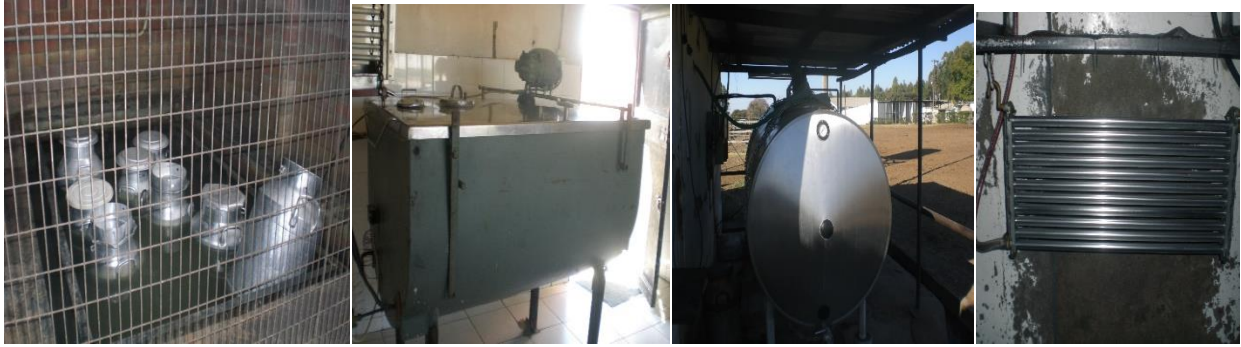
Figure 4.8. Various cold chain equipment from left to right, milk cans, open bulk cooler, closed bulk cooler and plate heat exchanger. Source: (Author, 2013)
