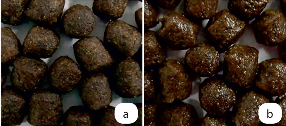
Fig. 1. Oil-coated pellet morphology for feed with 0 (a) and 200 g gluten  $\text{kg}^{-1}$  (b). Samples were coated using pilot-scale coater.
