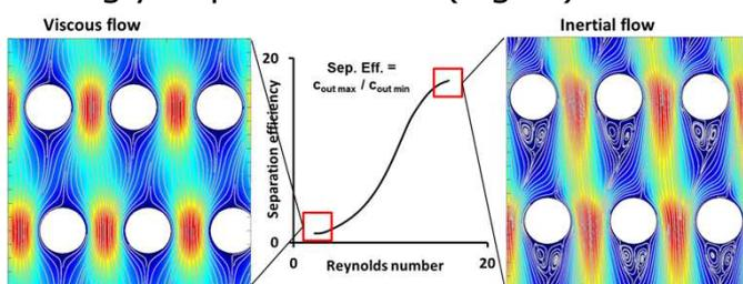
**Fig. 2.** Different flow regimes in deterministic ratchets lead to different separation behaviour<sup>2</sup>.
