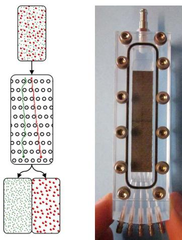
**Fig. 1.** Left: Separation by particle displacement in deterministic ratchets. Right: Ratchet device with a throughput of e.g. 9 L/h displacing particles in the range between 90 and 106  $\mu\text{m}$ .
