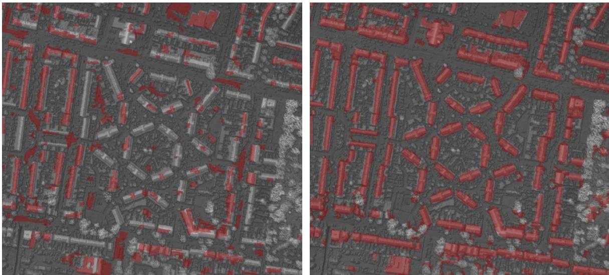
Fig. 40 Examples of spectral building feature extraction (left) and geometric building extraction (right). Building features are colored in red and superimposed over the hill-shaded reference surface.
