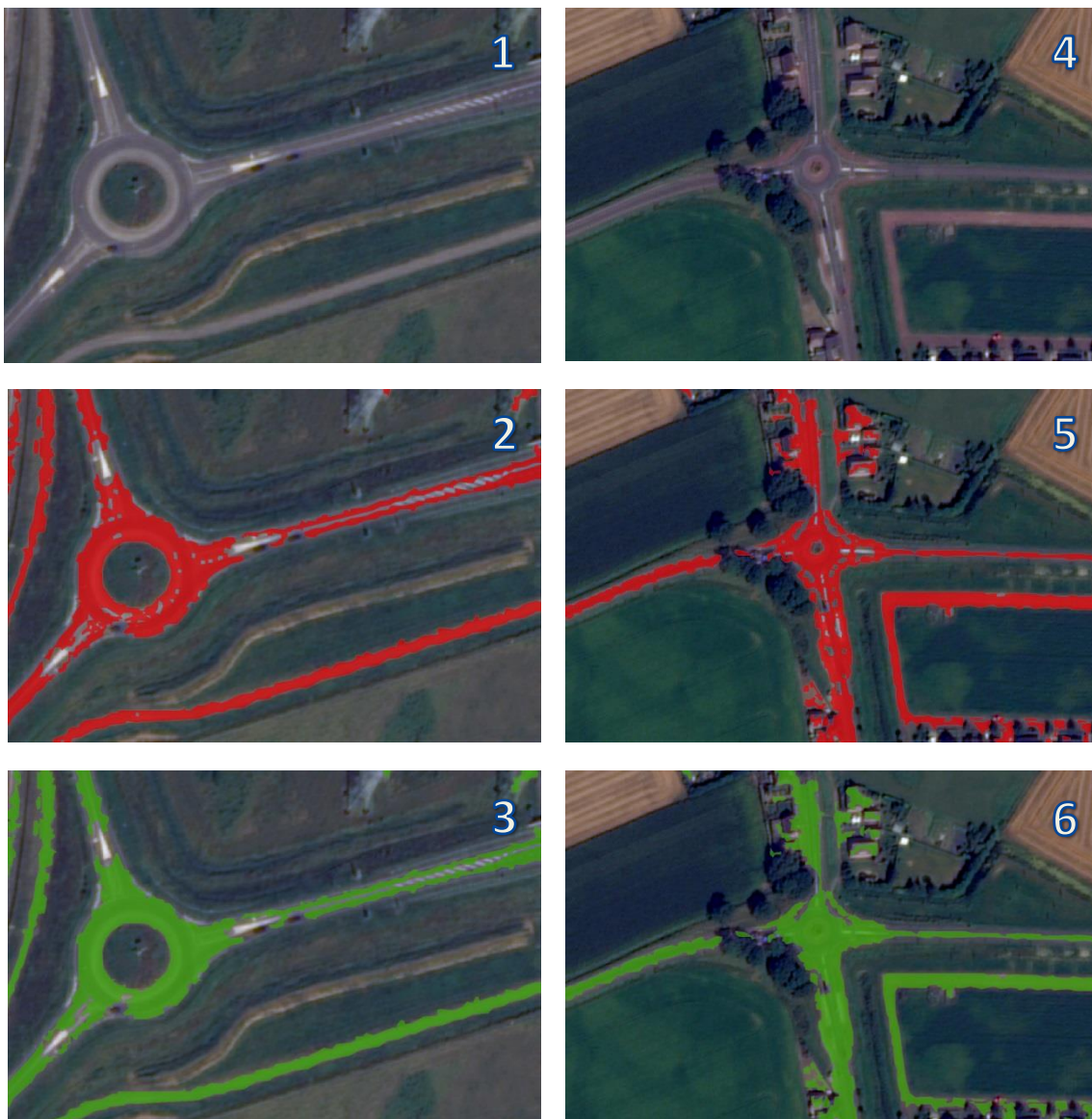
Fig. 44 Examples of successful (1-3) and unsuccessful (4-6) island filter operator implementation. Road features before implementation are colored in red, and after implementation in green.
