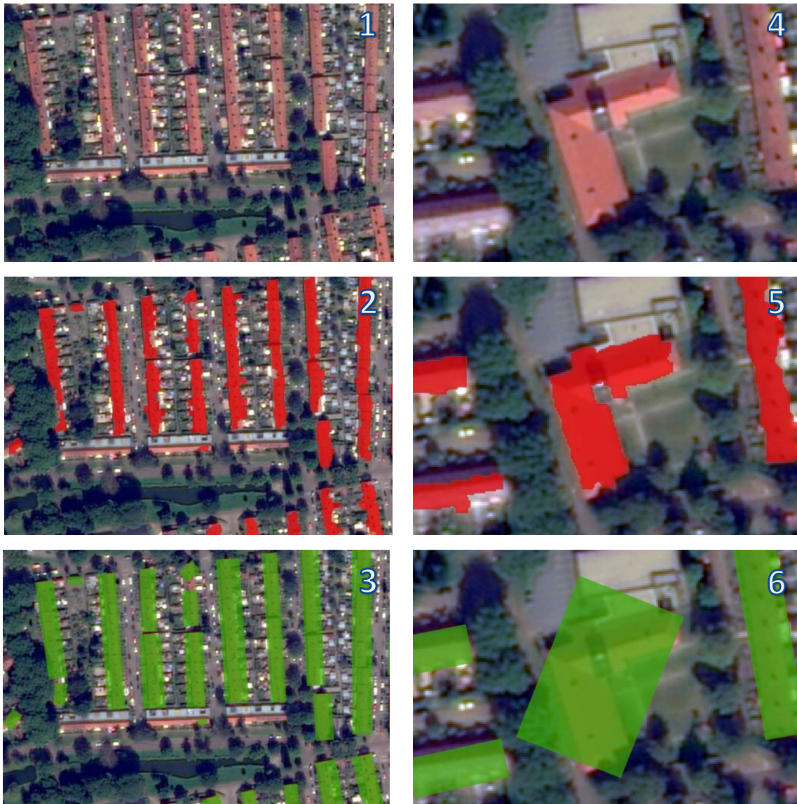
Fig. 43 Example of positive effects (1-3) and negative effects (4-6) of oriented bounding box operator implementation. Building features before implementation colored in red and after implementation in green.
