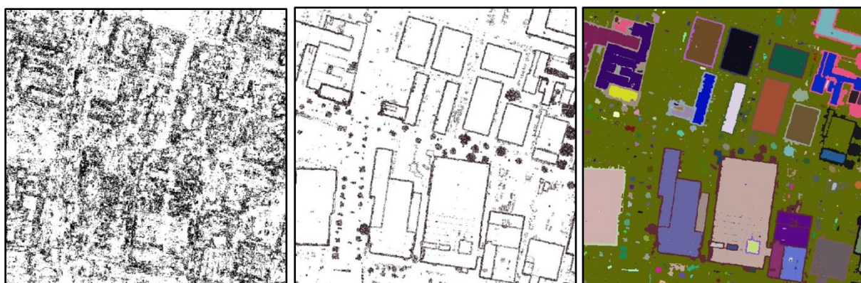
Fig. 25 Planar surfaces derived from photogrammetrically derived DSM (left), AHN2 LIDAR DSM (middle) and transformed AHN2 LIDAR DSM planar surface raster objects (right) in the Amersfoort study area.
