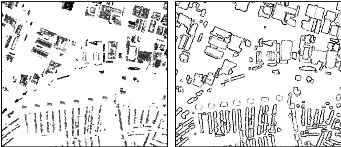
Fig. 49 Subdivided DSM (left: buildings and right: buffers) for extracted features and buffer zones.
