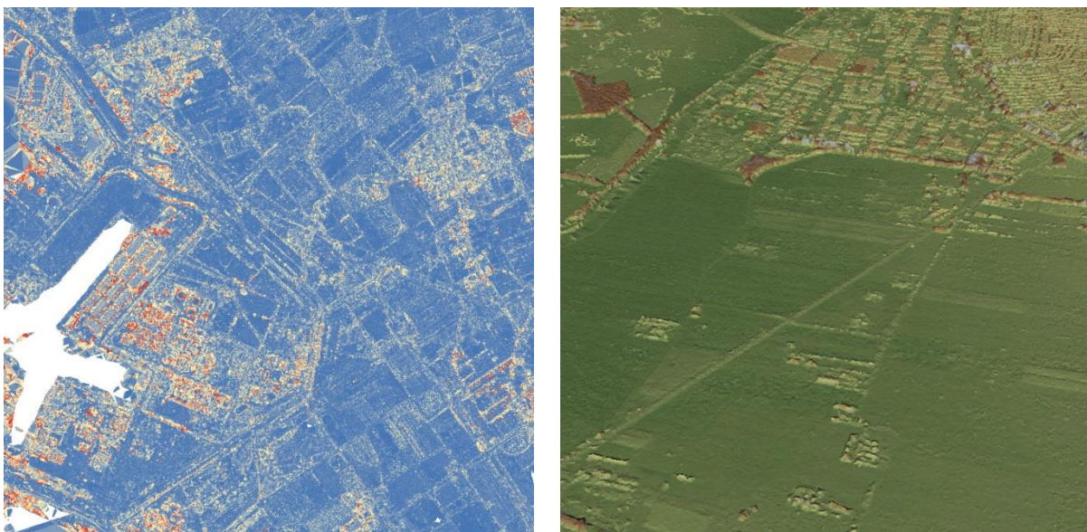
Fig. 30 Visual slope inspection over Vlissingen study site (left) and visual accuracy assessment over Amersfoort study site using TIN structures (right).
