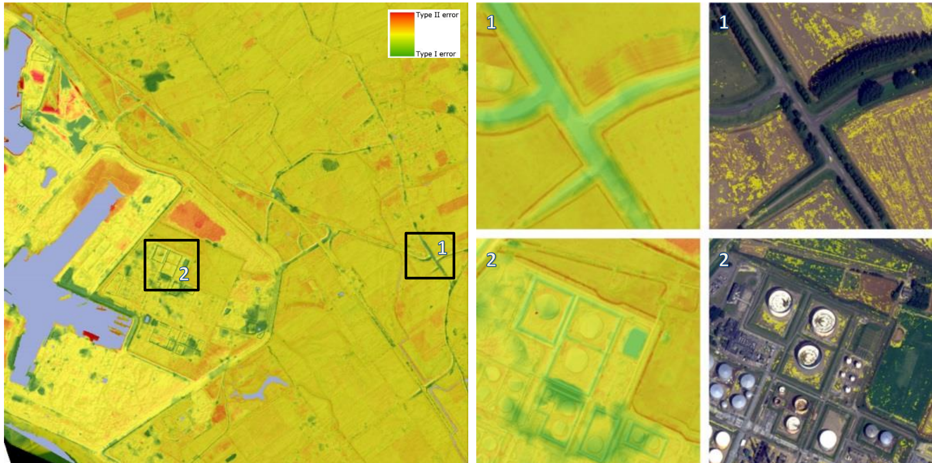
Fig. 54 Close-up examples of type I errors found in combined DSM to DTM filtering results at Vlissingen study site. Light green indicates the presence of type I errors. The non-interpolated bare earth points used for interpolation of the final DTM are colored yellow in the right column.
