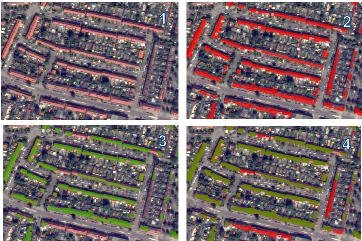
Fig. 47 Examples of errors in the pixel to vector domain conversion during feature extraction process. 1: orthorectified imagery, 2: building raster objects, 3: building vector objects, 4: building vector objects superimposed on building raster objects.
