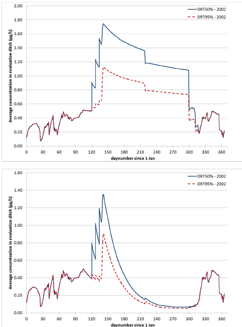
Figure 15 Tier-1 (upper panel) and Tier-2 (lower panel) exposure profiles for herbicide H_T on the basis of the new Dutch ditch scenario and 50% (blue line) and 95% (red line) drift reduction.
