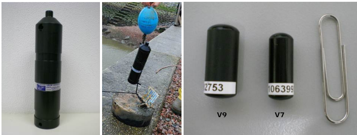
Figure 3.3.1. VEMCO VR2W receiver (left), receiver mooring with a float and a weight (middle), and VEMCO transmitters V9 and V7 (right).
