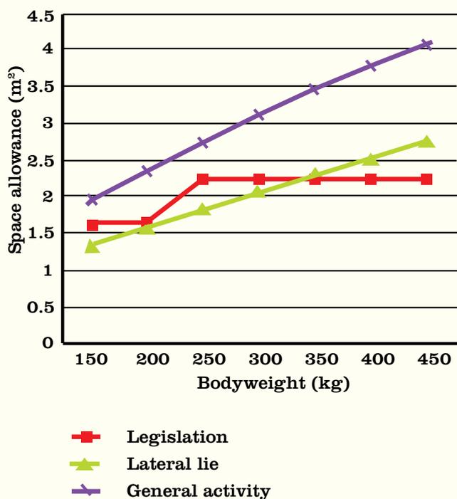
The space required for a sow to lie in lateral recumbency is given by the allometric equation  $A=kW^{0.67}$  where A is space in m<sup>2</sup>/animal, k is an empirical constant set at 0.0457 for lateral lying, and W is bodyweight. Extrapolation of the k value for general activity (of an animal in straw based systems with natural light) estimates k at 0.068 (see Information sheet 3 listed in references).
