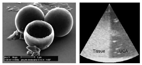
Figure 8. Hollow ultrasound contrast agent (taken from the work of Böhmer et al (2007), and an image from a movie that shows ultrasound contrast agent flaring up on the right side, the left side is a phantom tissue placed there to show the difference in behaviour. The movie was made together with Erasmus Medical Centre; courtesy of Klazina Kooiman and colleagues.
