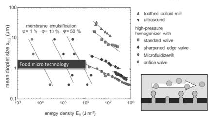
Figure 3. Comparison of various emulsification technologies based on energy density. The graph is adapted from: Schroeder, PhD thesis, TU Karlsruhe. Right bottom insert: principle of cross-flow membrane emulsification; the to-be-dispersed phase is pushed through the membrane and the droplets are sheared of by the cross-flowing continuous phase.
