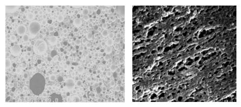
*Figure 5. Light microscopic images of milk (left), and a scanning electron microscopic image of a microfiltration membrane with nominal pore size of 0.2 micrometre (right).*
