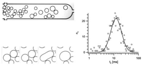
Figure 9. Microfluidic chip with a coalescence chamber for emulsion stability testing (top left image). Bottom left images show four consecutive images showing the coalescence process in detail. Right image, an example of a distribution of coalescence times as measured in the coalescence chamber (Krebs et al, 2012).
