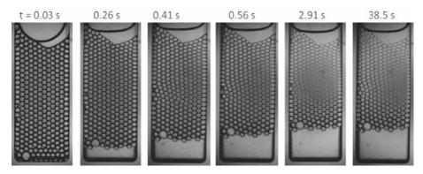
*Figure 10. Emulsion compression experiment carried out with a microchip place on a centrifuge (Krebs et al, 2013).*
