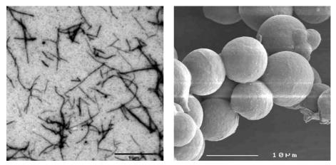
*Figure 7. Whey protein fibres produced at low pH (left image) and capsules made by layer-by-layer adsorption of highly methylated pectin and whey protein fibres; total amount of layers is 10 (right image) (Rossier Miranda et al, 2010).*
