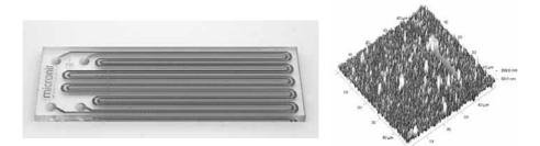
*Figure 11.* Copper containing microchip for emulsification (left image), and a roughness plot obtained by atomic force microscopy of the same surface (right image) (Maan et al, 2013).
