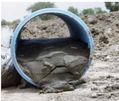
Figure 66 Plastic corrugated collector pipe half full with sediment (example from Pakistan)
