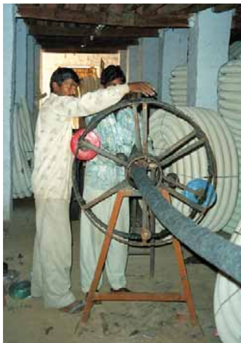
Figure 6 Wrapping the non-woven polypropylene envelope around the drain pipe
