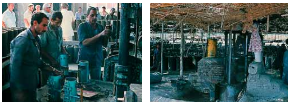
Figure 8 Concrete pipe factory in Tanta in the Nile Delta (a) and a mobile production unit in a field workshop, where concrete pipes are stored in a shaded area (b)
