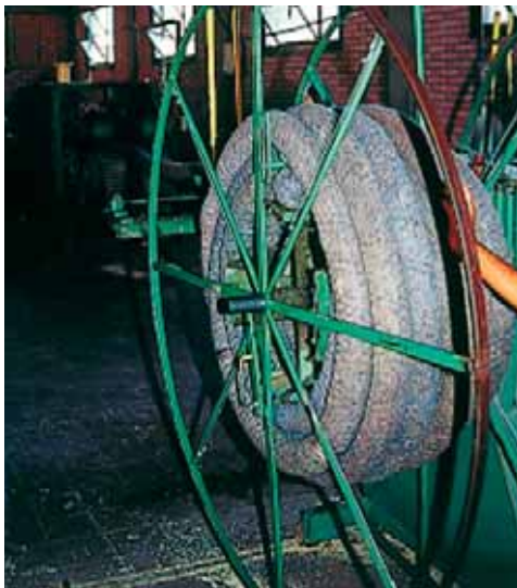
Figure 10 PVC pipes are pre-wrapped with a voluminous envelope in the factory in Tanta
