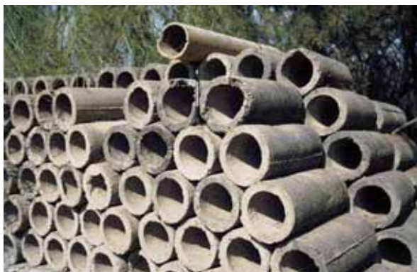
Figure 2 Concrete pipes (Ø 100 mm) used in Sampla Pilot Area, Haryana
