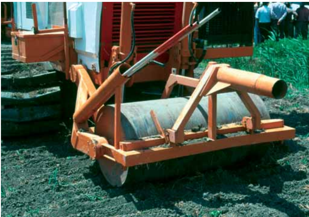
Figure C12.2 Roller in front of trenchless drainage machine
