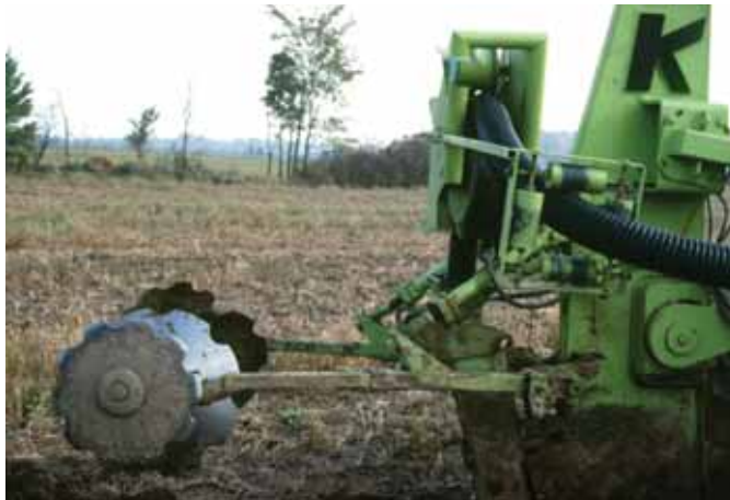
Figure 47 Backfill equipment: tractor with dozer blade (a) and V-shaped disc-blade mounted at the rear end of a subsoiler type trenchless drainage machine (b)
