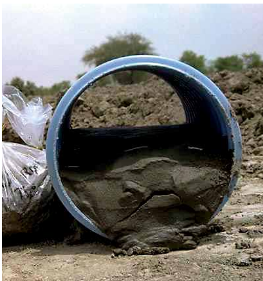
Figure 9 Fourth Drainage Project: excavations revealed that the drain pipes were blocked by fine sediments
