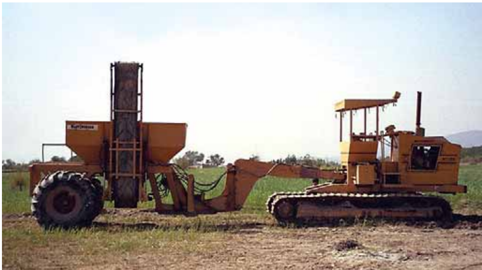
Figure 8 Track-mounted gravel feeders and gravel trailers with float tyres for maximum bearing were used in the Chashma CAD Project
