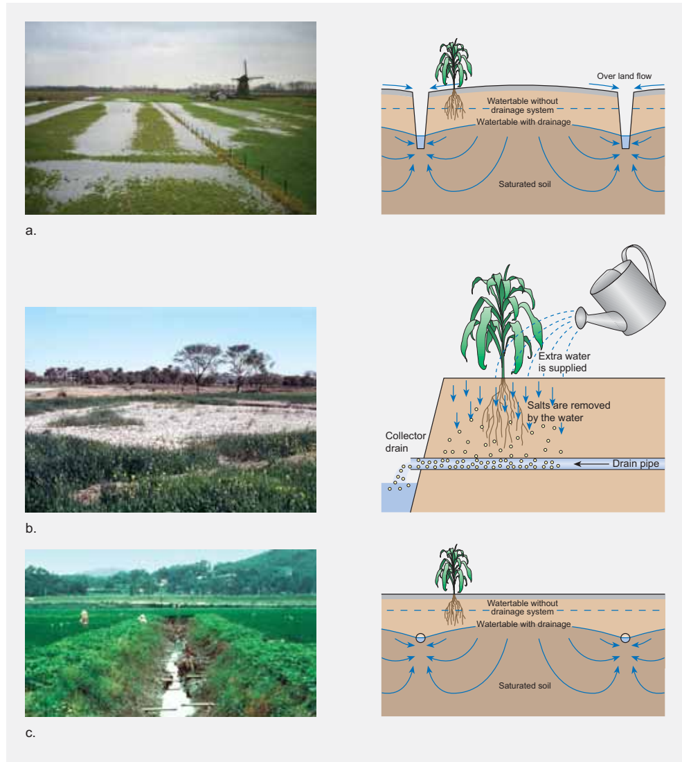
Figure 1 Objectives of drainage are: (a) to remove excess water, (b) to control salinity and (c) to maintain the watertable at a desired level
