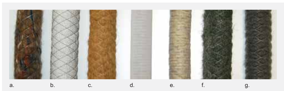
Figure 25 Envelopes can be made of wrapped polypropylene fibres (a, f & g), polystyrene granules (b) and coconut fibres (c), non-woven nylon (d) and woven tyvar (e)
