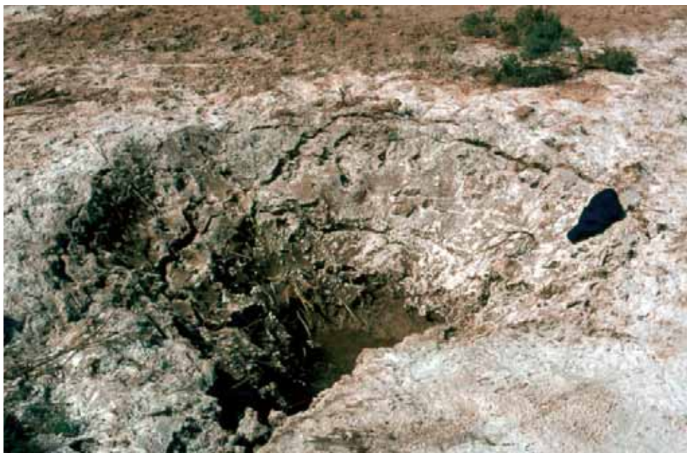
Figure C33.2 Erosion ("piping") of unconsolidated trench fill
