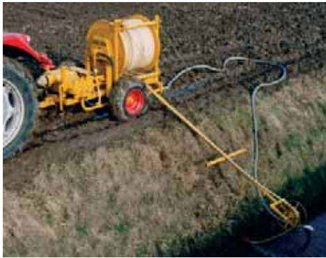
Figure E2.1 A high (left) and medium (right) pressure flushing machine
