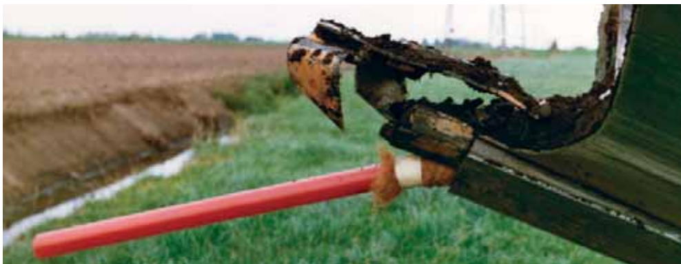
Figure C10.3 Iron flap with knives at the rear end of the V-plough
