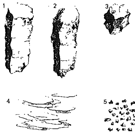
Figure 3.3 Drawings illustrating some types of structural elements (at different scales): 1) prismatic, 2) columnar, 3) blocky, 4) platy, and 5) granular (Soil Survey Staff 1975)
