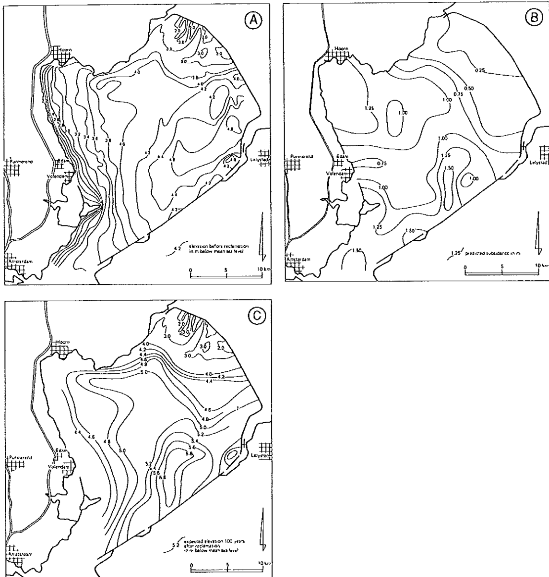
Figure 13.17 Elevation of the soil surface of the Markerwaard area A: Before reclamation; B: The predicted subsidence; C: The expected elevation 100 years after reclamation (Ente 1976; Van der Scheer 1975)
