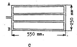
10 mm.). Tube ABC is bent as shown on the figure, C being the highest point of the drain. Nylon cloth ribbon is wrapped around the drain in such a manner that a covering is obtained consisting of three layers of nylon cloth. Washing beforehand in T-ppl is recommended as to remove all traces of dres-
