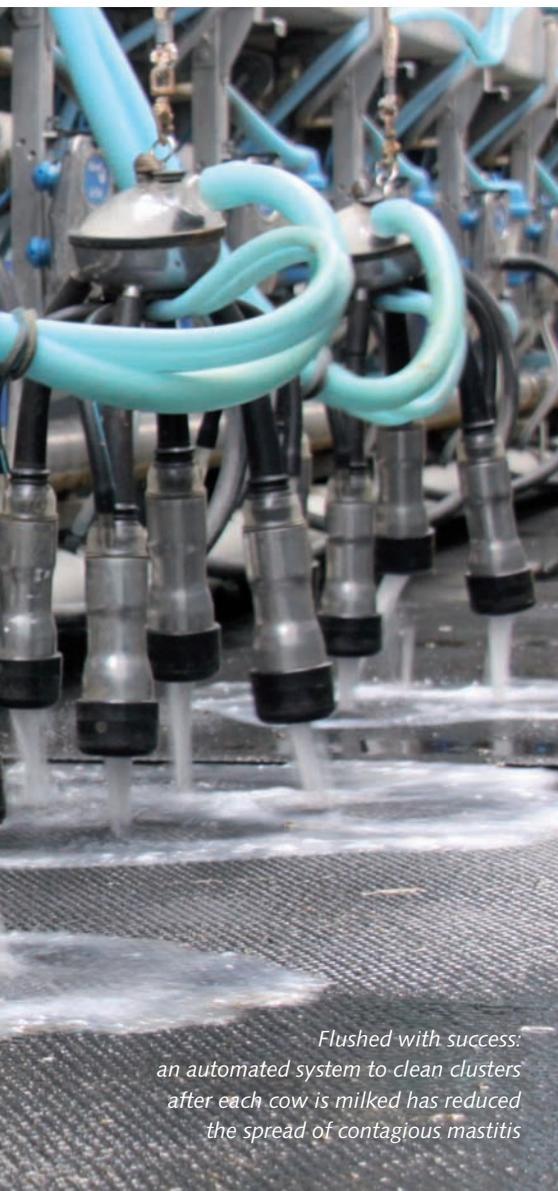
*Flushed with success: an automated system to clean clusters after each cow is milked has reduced the spread of contagious mastitis*
